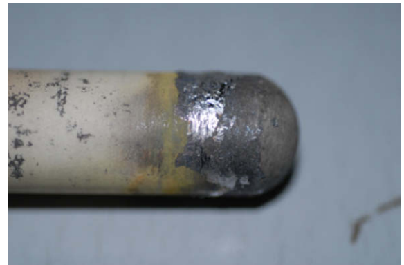
Fig. 9. Appearance of the YSZ surface of the Pt/gas reference sensor after test 4 in LBE.
