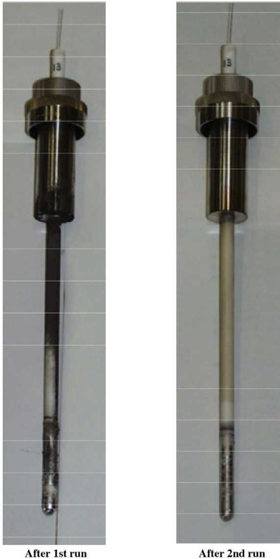
Fig. 7. Photos showing appearance of the Mo/Bi-Bi 2 O 3 reference sensor after measurement in LBE.
